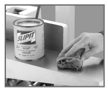
Figure 43. Applying lubricant to table surface.
